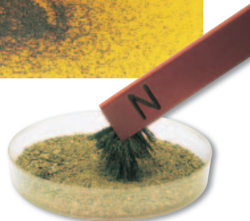
Magnetism easily separates iron from sand.
