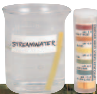
Figure 10 The pH of a sample can be measured in several ways. Indicator paper gives an approximate value quickly, however, a pH meter is quick and more precise.
